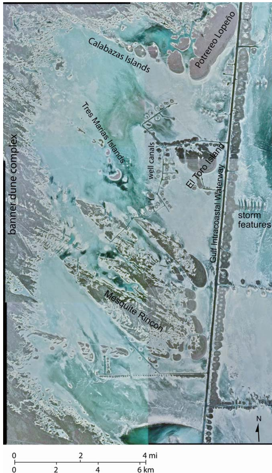
Figure 2. 1996 aerial photograph showing the natural and man-made geomorphic features of the wind-tidal flats of Laguna Madre. Location shown in Figure 1 .
